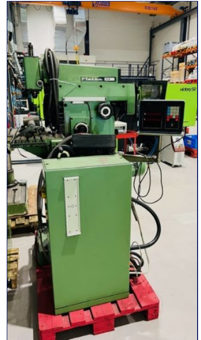
Fresadora universal 600x210 mm METBA MB-1 Ref: ITM-001
