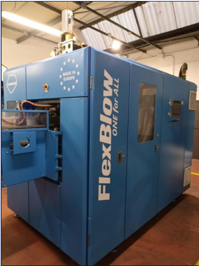
Sopladora botellas PET 6 litros TEREKAS FLEXBLOW 2 Ref: GST-001
